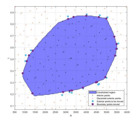
The **Maximum boundary points (% of points)** option limits the maximum number of boundary points as a percentage of the total number of design of experiment (DoE) points. The total number of DoE points is equal to the number of interior points plus boundary points. For example:
